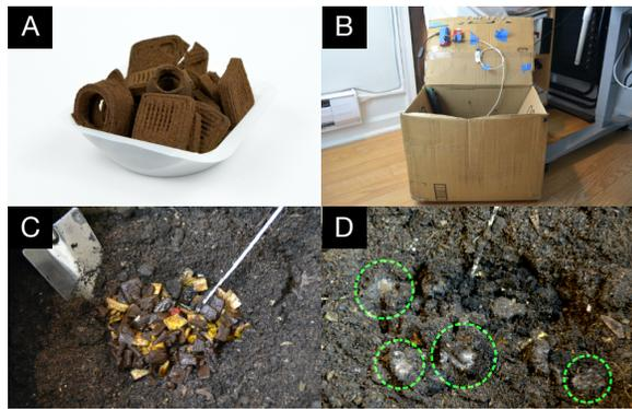
**Figure 7: Composting of SCG Material.** Objects made with our SCG material (A) can be inserted into a compost box at home (B) with other food scraps (C). Within a few days, microorganisms like mold grow and begin breaking the material down into compost (D).
