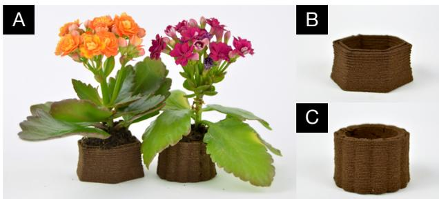
**Figure 12: Planter pots** printed with our SCG material and their flowering plants (A). The first pot (52 mm x 60 mm x 36 mm) has a hexagonal-shape (B). The second pot (48 mm x 49 mm x 40 mm) is cylindrical with a ribbed pattern (C).
