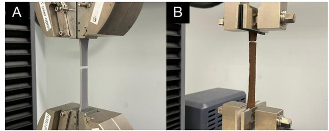
**Figure 5: Experimental apparatus for the ASTM standard D638-14 tensile strength test comparing PLA (A) to SCG material (B).**
