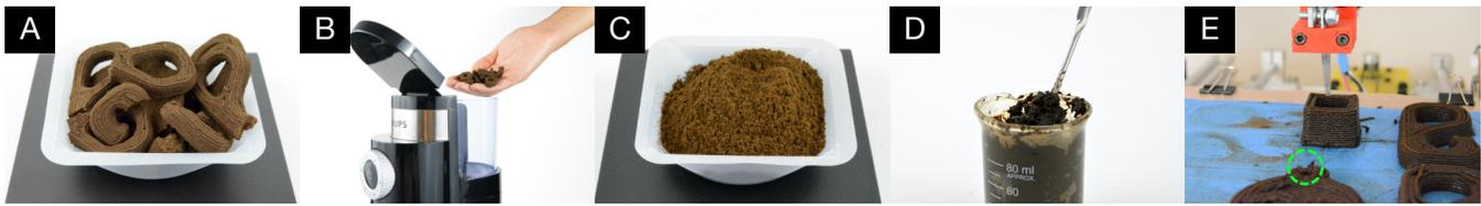
**Figure 10: Material Recycling Workflow.** Objects printed with our SCG material such as prototypes and failed prints (A) can be ground up using a basic coffee grinder at home (B). The resulting granules (C), once weighed, can then be mixed with a proportional amount of water (D) to produce our SCG material again for printing (E). This recycling approach is useful in minimizing waste when a printing error unexpectedly occurs such as a gap in extrusion (green circle).
