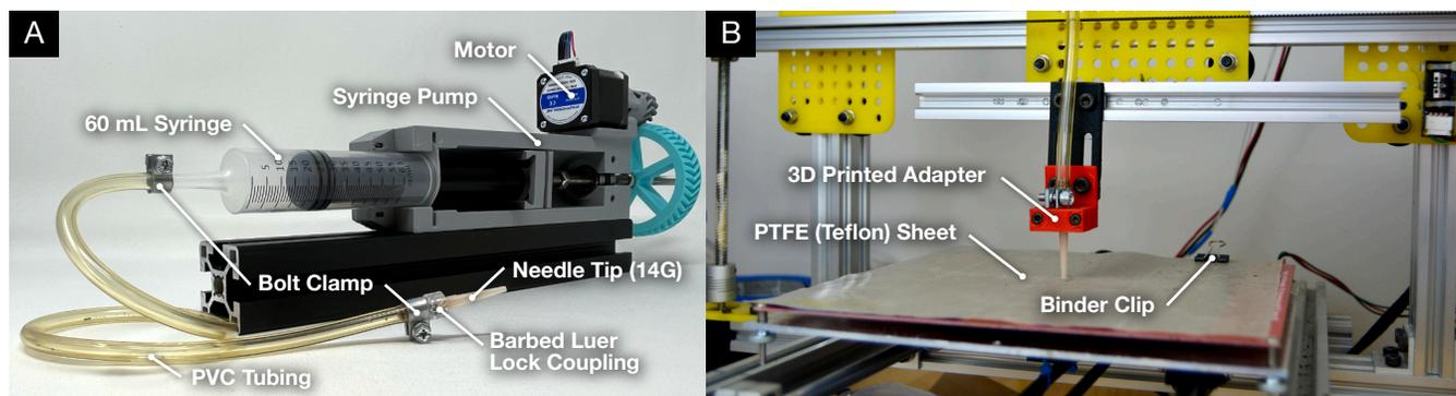
Figure 3: The extrusion set-up and components (A) used to print our SCG material on a modified FDM/FFF 3D printer (B).
