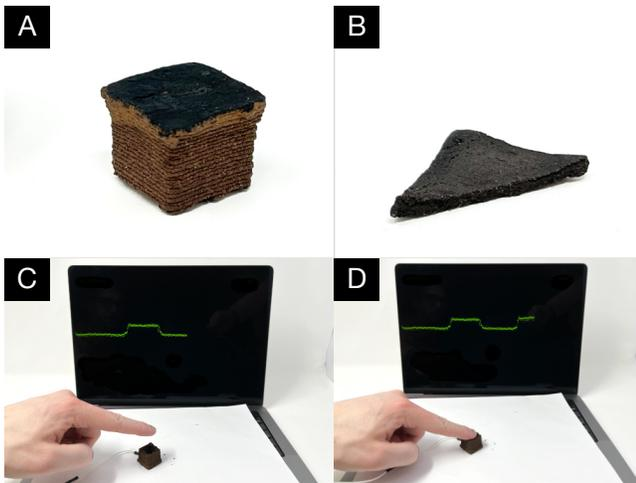
**Figure 14:** Two capacitive sensors made from the SCG material and activated charcoal powder: a hollow cube (A), and a cast triangle (B). The conductivity in the material provides touch-sensing capabilities as a finger touches the surface of an object (B,C).
