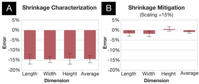
**Figure 4: Shrinkage characterization and mitigation for our SCG material. The average error in dimensional accuracy for five printed specimens (30 mm x 30 mm x 5.6 mm) once dried is -14.53% (SD=1.94) (A). After uniformly scaling the geometry of specimens by 15.0% before printing, the average error in dimensional accuracy caused by shrinkage for five printed specimens reduced to -1.05% (SD=0.60).**
