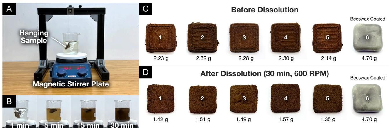
**Figure 6: Water dissolution test set-up and results for six SCG material specimens. (A) An SCG material sample is suspended with monofilament fishing line inside a beaker containing 150 mL of water. (B) The water is agitated at 600 RPM using magnetic stirrer plate for 30 minutes to progressively dissolve the material. The visual quality and mass (g) of six specimens (five consisting of only SCG material and a sixth is coated in beeswax) before (C) and after (D) the test are shown.**
