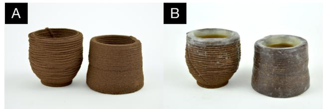
**Figure 13: Compostable espresso cups** made from SCG material (A). The left cup is 57.8 mm x 57.8 mm x 55 mm and the right cup is 57.8 mm x 57.8 mm x 49 mm. The cups hold liquid once beeswax is applied either on the inside of the cup (B, left) or around the cup entirely (B, right).
