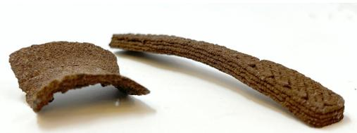
**Figure 15:** Two objects printed with our SCG material that changed their shape as they dried: a flat square morphed into a saddle shape, and a rectangular rod bent upwards as a result of shrinkage during drying.
