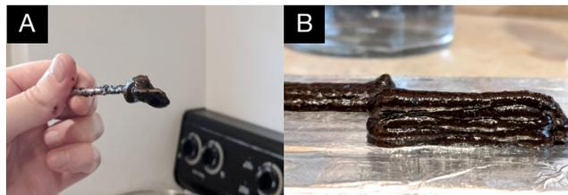
**Figure 2: Determining suitable thixotropy.** We found when the SCG material holds its shape on a stirring rod and does not drip (A), it is self-supporting and exhibits thixotropic behavior suitable for hand-extrusion and 3D printing (B).
