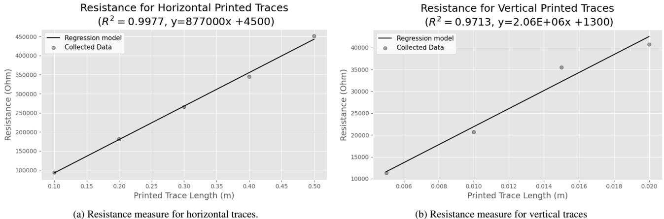
Figure B.1: The two linear regression models informed how to generate (i.e., draw) the conductive traces for fabrication (Sect 3.5) such that it achieves the resistance optimization (Sect 3.3.2).
